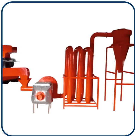
(8.3) MATERIAL DRYING SYSTEM
